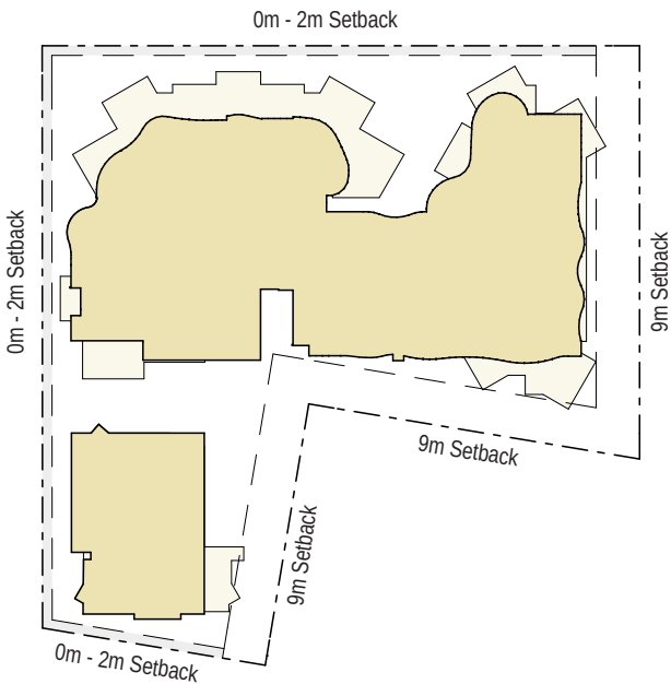
Concept Plan - Proposed Ground Floor Setbacks
